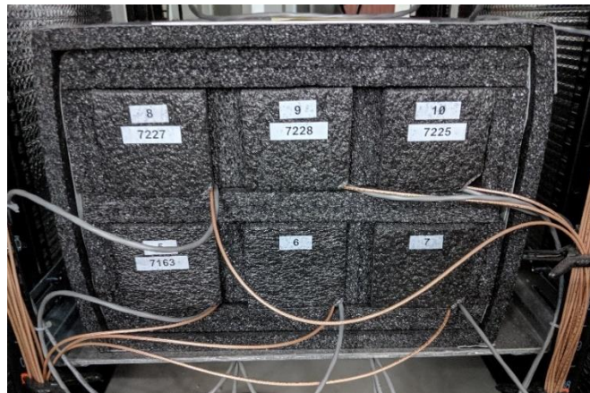
Figure 21: MMS setup – insulated OCXOs
