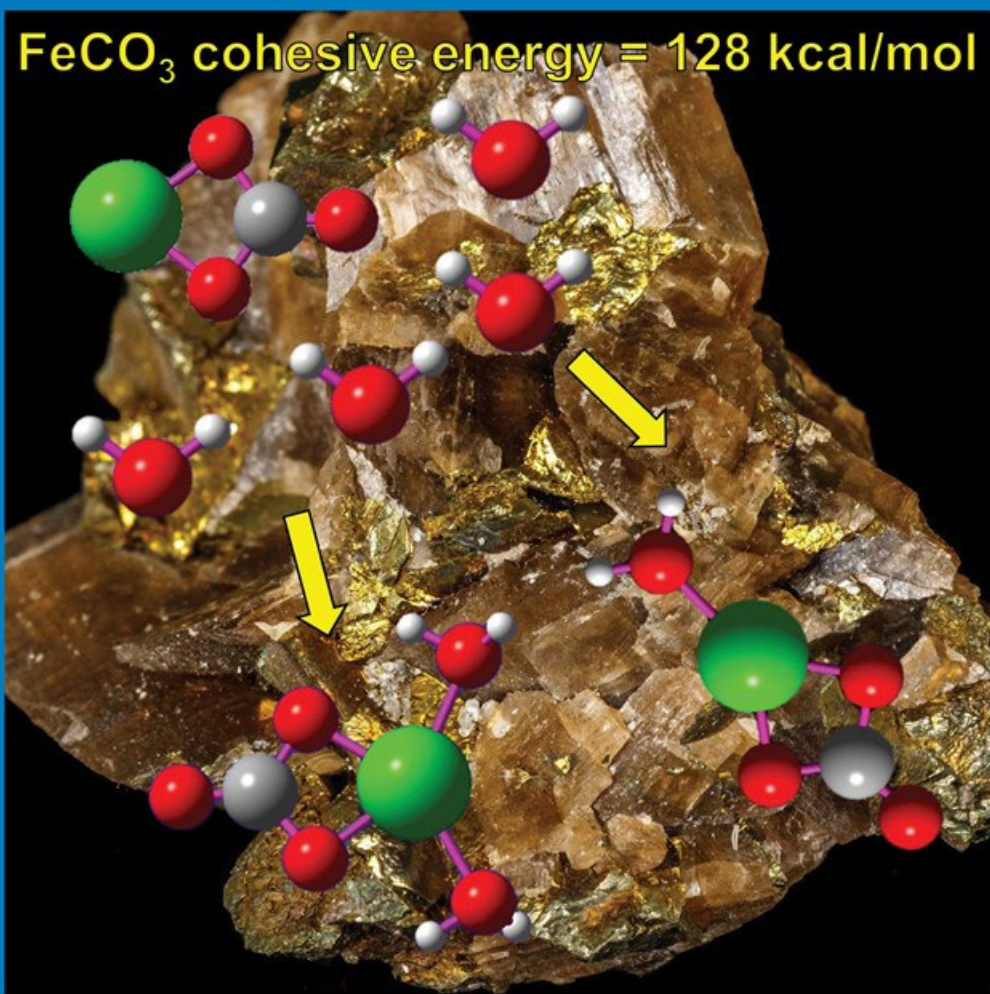
Figure 7.1. Cohesive energy of \text{FeCO}_3 at 298 K in kcal/mol and hydrated structures of \text{FeCO}_3 . Green atoms = Fe, red atoms = O, grey atoms = C and white atoms = H.
