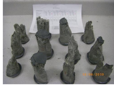
Fig. 2. Specimens with Capping Fig. 3. Setup of Strength Testing Fig. 4. Specimens after Testing
