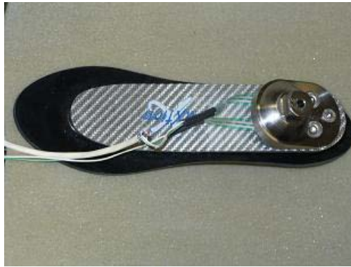
Figure 4.4 Instrumented prosthetic foot with force resistors
