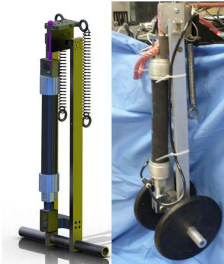
Figure 5.7 Actuator computer model and completed bench-top tester
