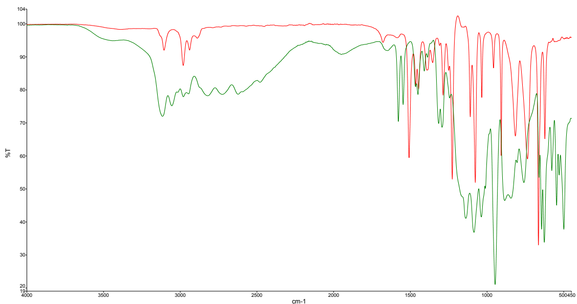
Figure 8.6.12: FTIR spectra for 1,2-diethyl-4-methylimidazole sample: neat (red) and \text{SO}_2 -loaded (green).
