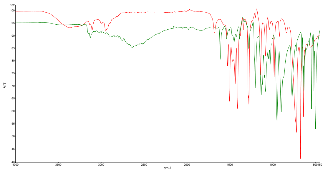
Figure 8.6.13: FTIR spectra for 1,2-dimethylimidazole sample: neat (red) and \text{SO}_2 -loaded (green).
