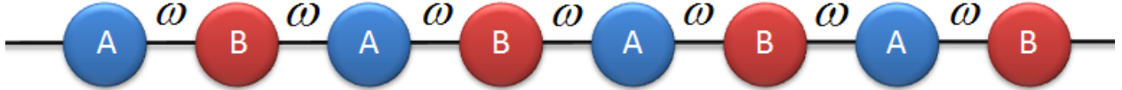
Figure 3.1. 1D atomic system with two sub-lattices. type A atom sits on one sub-lattice and type B atom sits on the other. There is only nearest neighbor interaction and the interaction is represented by the hopping parameter \omega .
