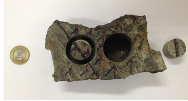
Figure 10. Core extraction from oriented sample for AMS analysis. Blue arrowhead showing dip direction in sample.
