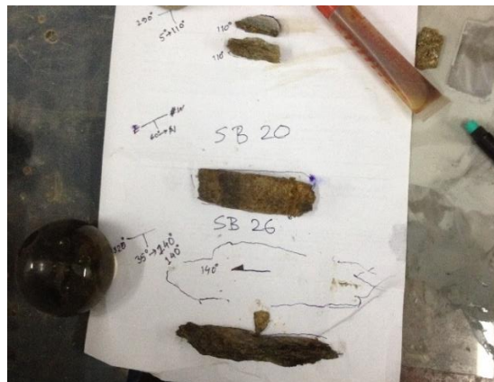
Figure 8. Method of transferring dip direction of foliation on thin section before polishing. Arrowhead towards top of the sample.
