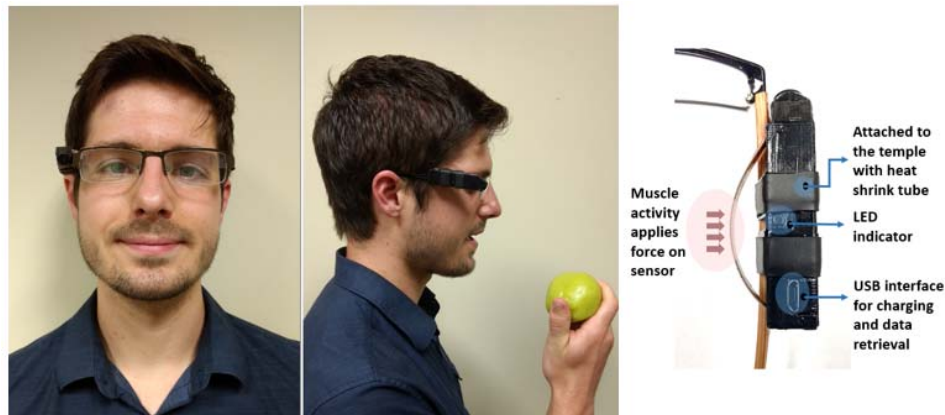
Figure 6-1. AIM-2 used to monitor chewing activities and capture passive images. The sensor module is attached to the temple of off-the-shelf wearable eyeglasses with heat shrink tubes.
