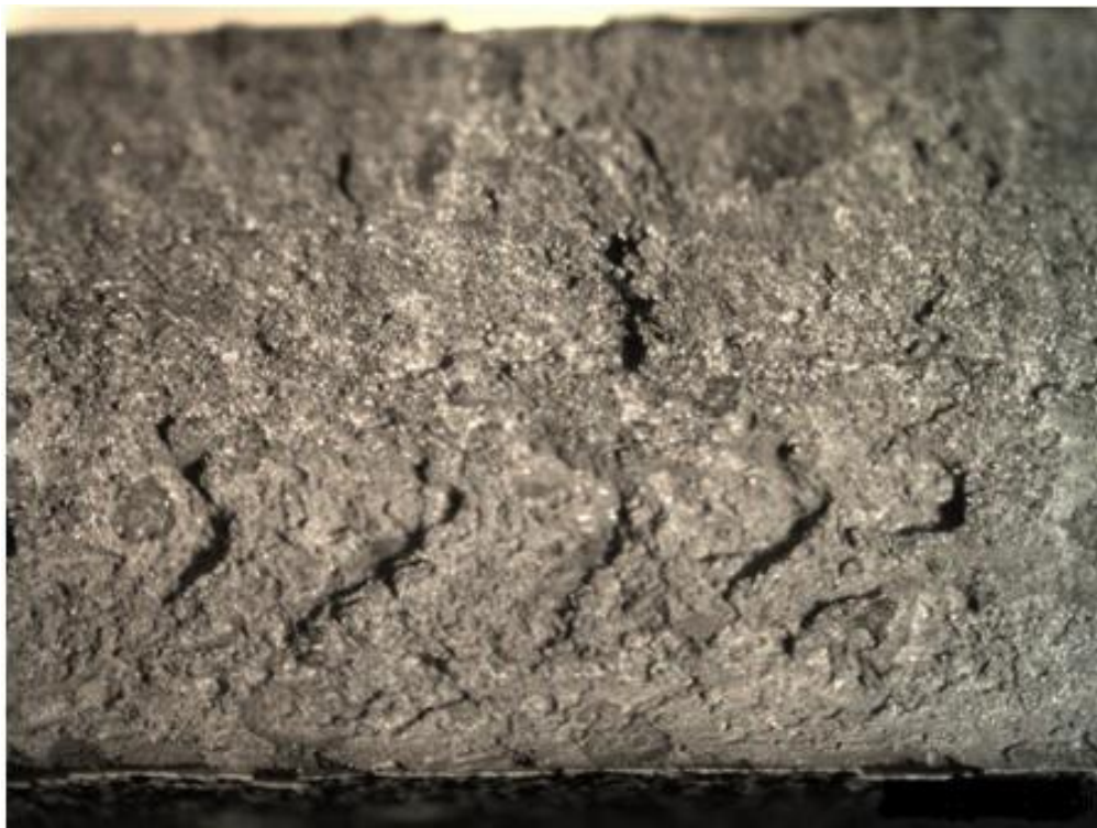
Figure 3.41 Ductile fracture surface of SR-FSW.
