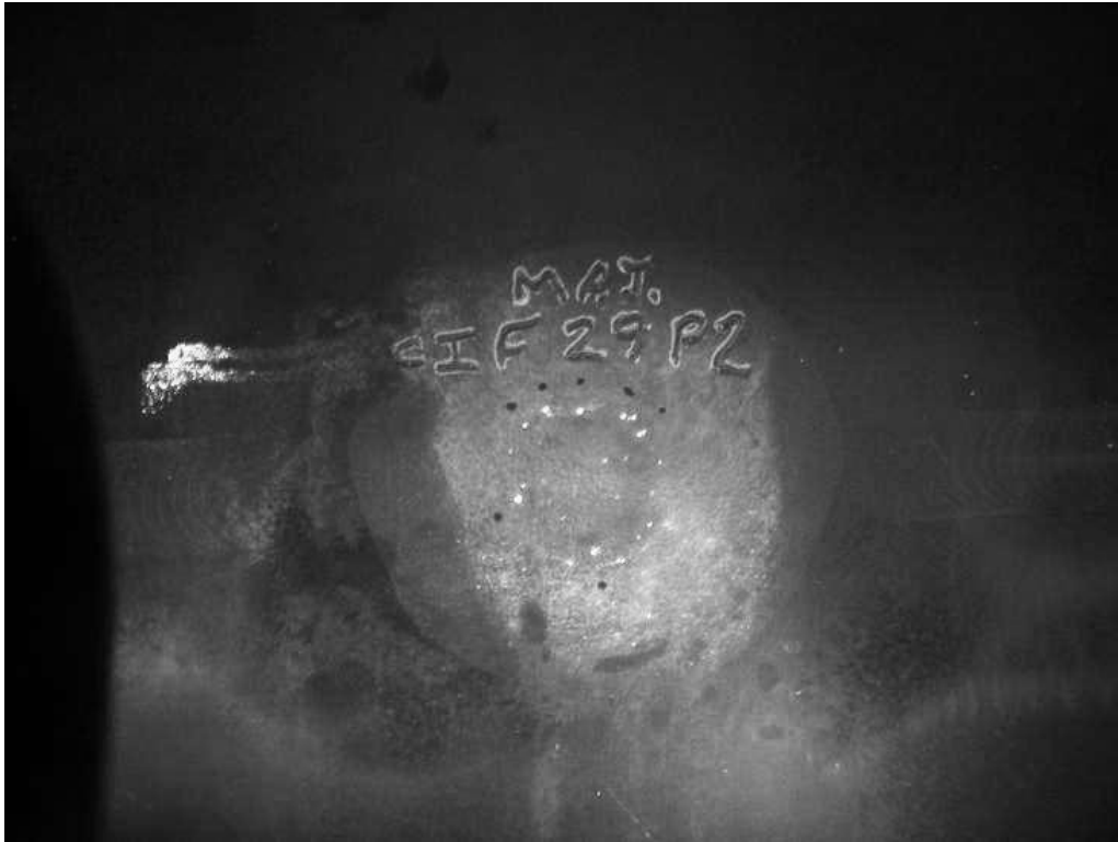
Figure C5 Round indications marked with red marks.
