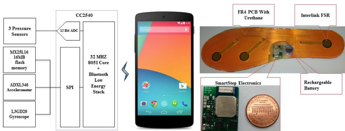
Figure 3-1. SmartStep block diagram and fully encapsulated insole.
