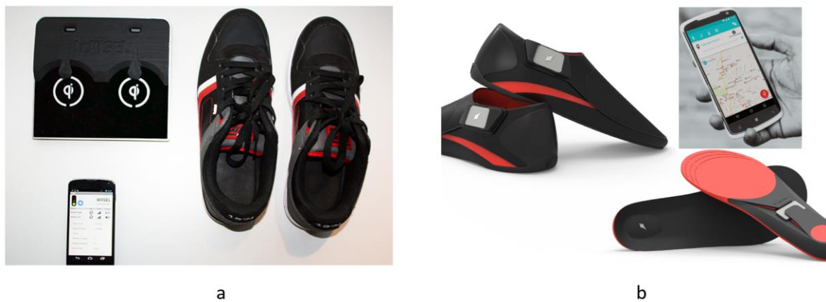
Figure 2-5. (a) Wiisel footwear system for fall risk application; and (b) Lechal system® for by Ducere Technologies pvt. ltd.
