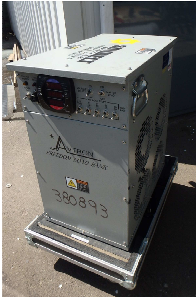
Figure 7-5. Avtron Freedom load bank and Shark® 100 power meter.
