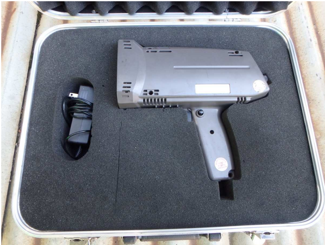
Figure 7-7. Image of the DT-725 stroboscope used to measure engine speed.
