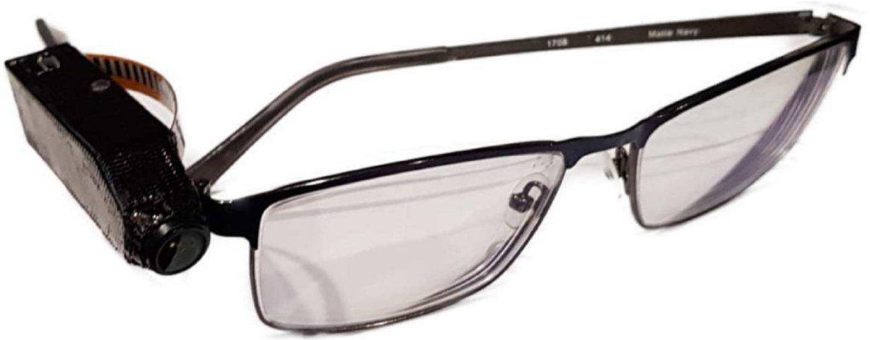
Fig. 4. AIM-2, an egocentric wearable camera with food intake detection sensors.
