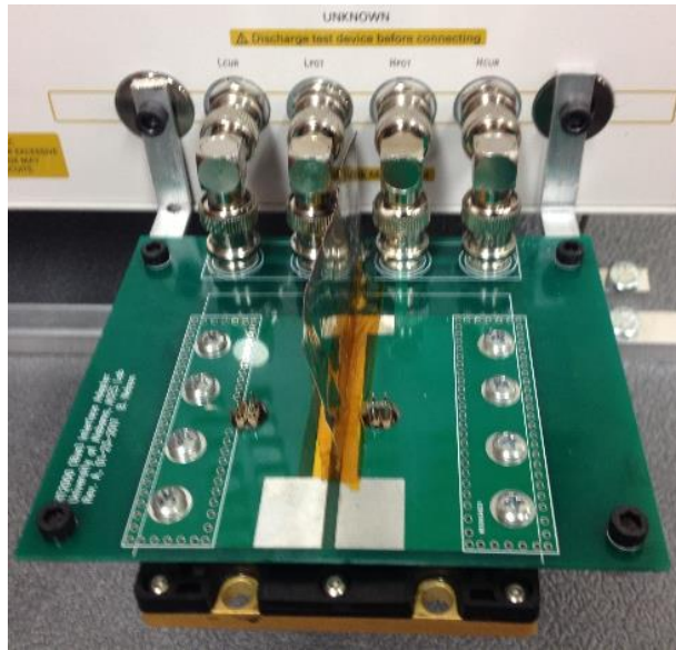
Figure 19: Bus+ to Bus- Interface Board
