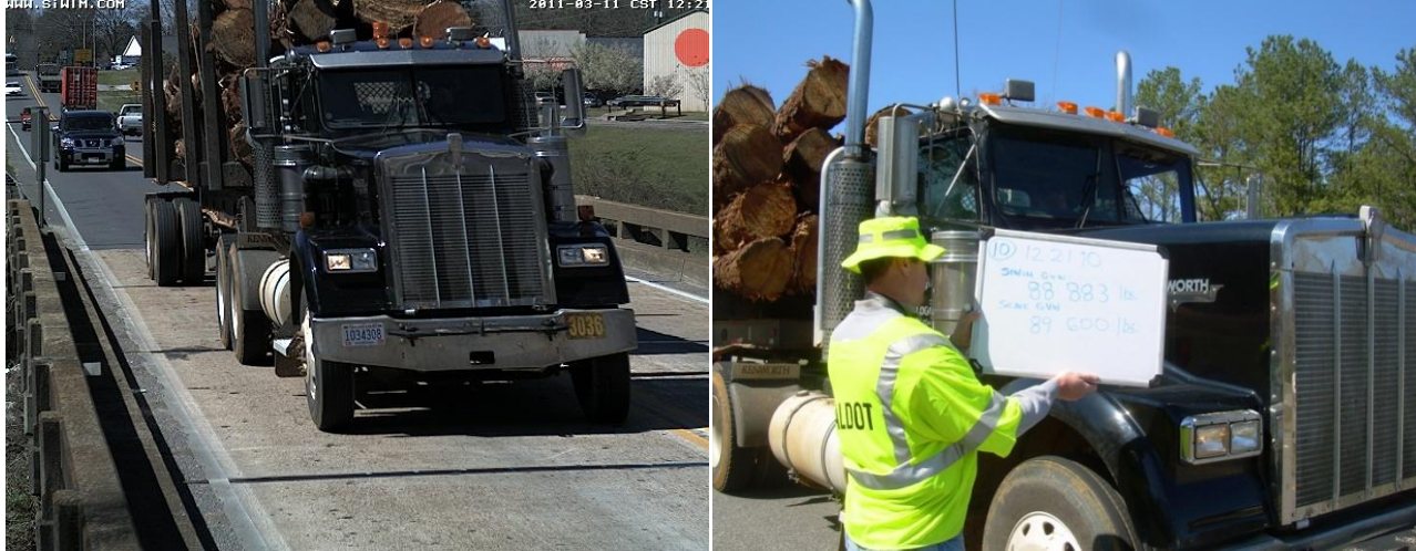
Figure 5.6 Photo of pre selected truck from SiWIM/Photo of truck being statically weighed
