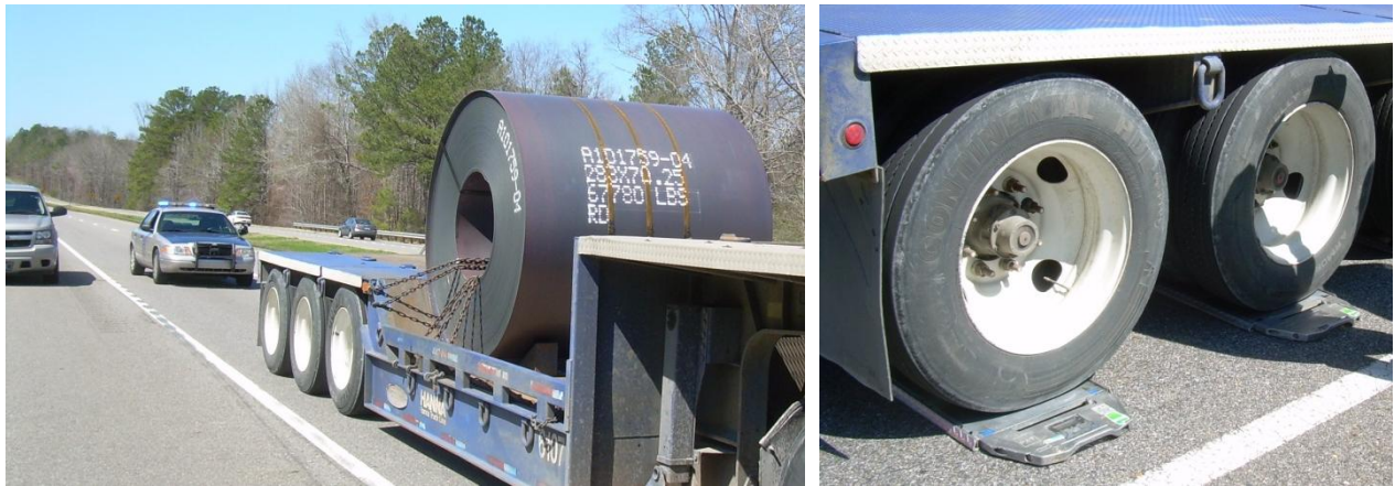
Figure 3.17 State Trooper puling over pre selected truck/Static weighing of truck
