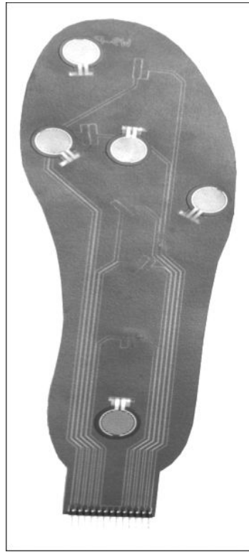
Figure 1b. Close-up view of flexible insole with embedded force sensitive resistors.
