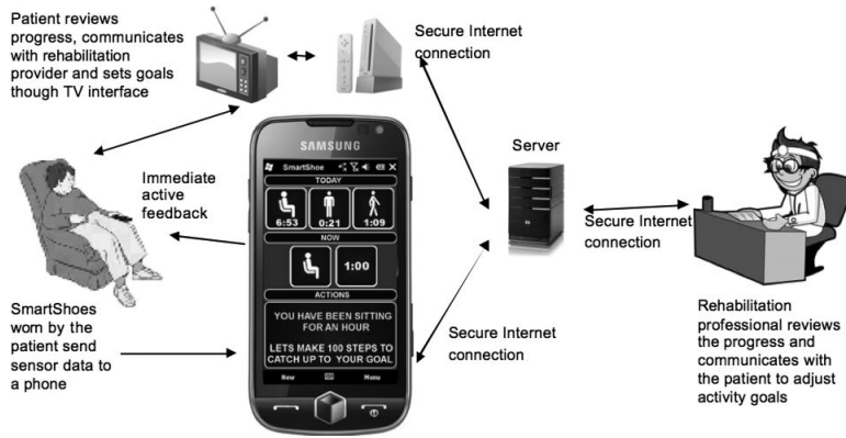
Figure 4. Mobile health concept using the SmartShoe as a method to self-monitor activity levels and receive real time feedback to promote increased activity levels.
