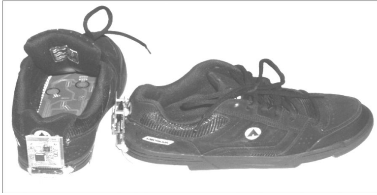
Figure 1a. SmartShoe sensor system with accelerometer, battery, power switch and wireless board on the back of shoe with the flexible insole with embedded force sensitive resistors.
