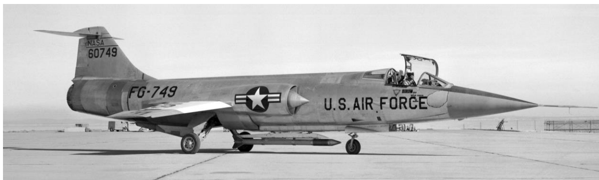
Figure 2-2. F-104A Starfighter shown with the Air Launched Sounding Rocket (ALSOR) attached on December 16, 1959 ("Air Launched Sounding Rocket (ALSOR) Attached to F-104," 1959).
