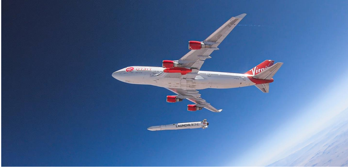
Figure 2-3. Virgin Orbit completing a drop test of LauncherOne on July 10, 2019. (Russell, 2019)
