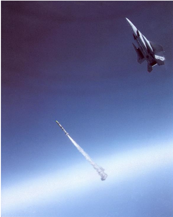
Figure 1-1. Successful launch of an anti-satellite, or ASAT, missile from a highly modified F-15A Sept. 13, 1985 scoring a direct hit on a satellite orbiting 340 miles overhead. (Reynolds, 1985)
