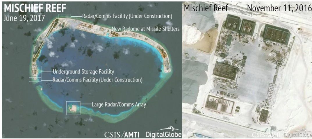
Figure 4-11. Artificial island, Mischief Reef, build-up including SAM batteries, radar, communications, and EW capabilities ("A Look at China's SAM Shelters in the Spratlys," 2017; "Updated: China's Big Three Near Completion," 2017). SAM batteries under-construction are shown on the right.
