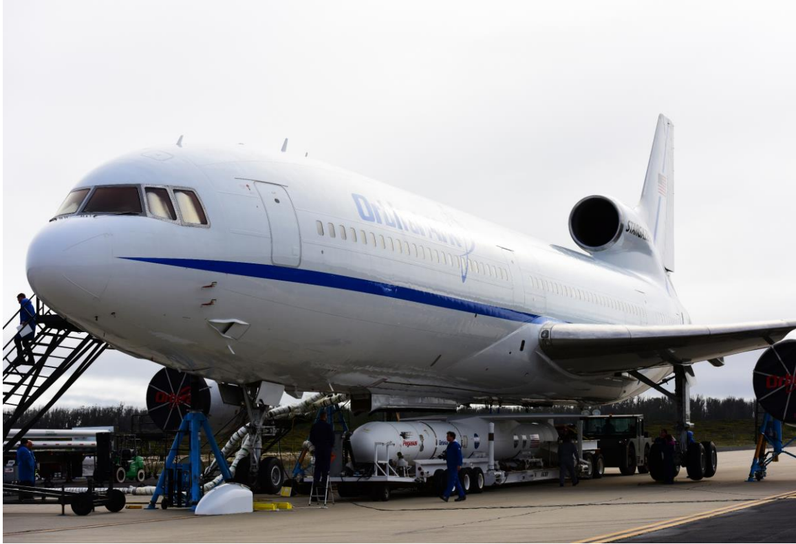
Figure 2-4. The Pegasus XL being mated with the Orbital ATK L-1011 aircraft to launch CYGNSS (Herrera, 2016).
