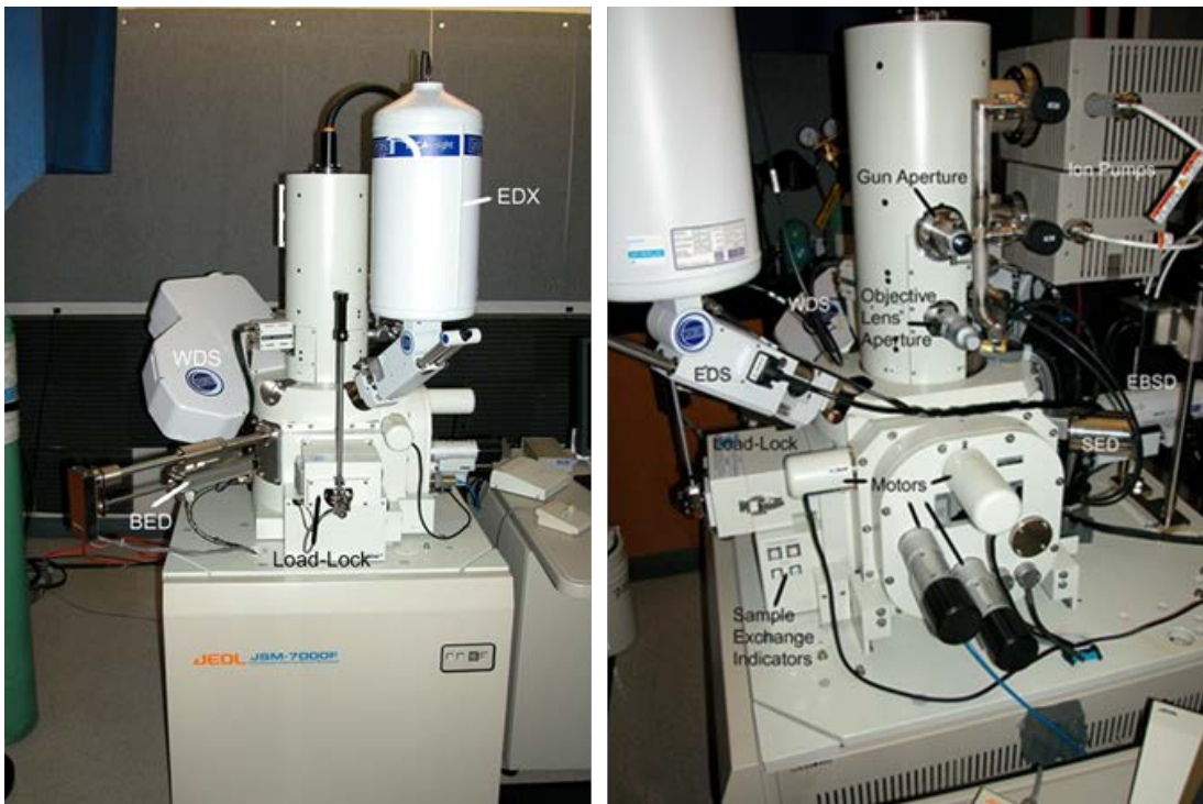
Figure 2-2: JEOL 7000F SEM, front and side view and labelled all the detectors
