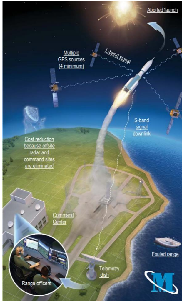
Figure 1. AFTS Concept Diagram (Valencia, 2019). AFTS does not utilize human-in-the-loop or over-head satellites for telemetry relay.
