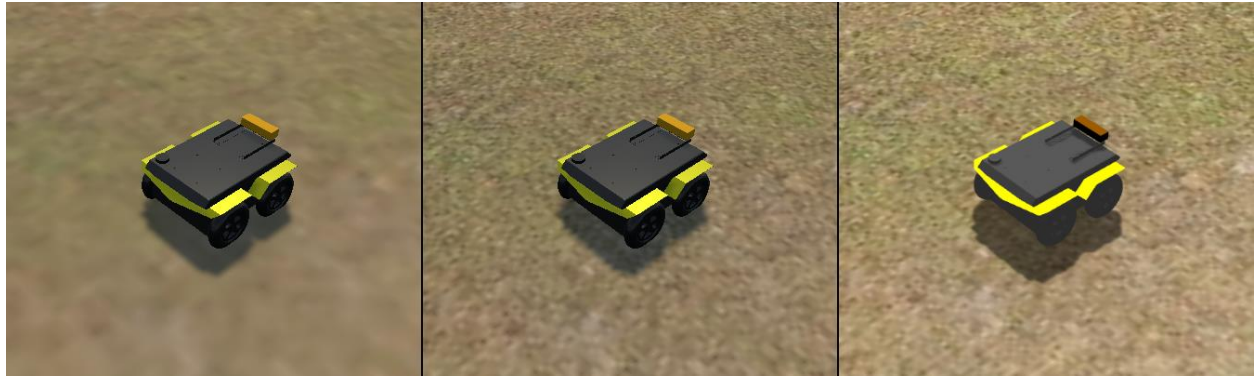
(a) (b) (c) Figure 25. Close-up comparison between textured landscapes (a) Unity3D at default import resolution, (b) Unity3D at full import resolution, and (c) Gazebo reference.
