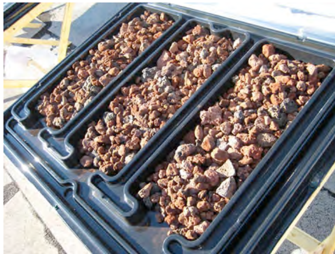
Figure 10.2.2 Rigid acrylic panel with rock filled basin
