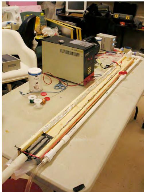
Figure 2.3.4 Unsuccessful attempt using magnetic force over an open race
